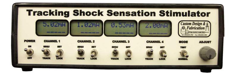
The Shock Sensation Stimulator is an effective tool for behavioral modification. The device utilizes an isolated and regulated alternating current source to provide a safe yet effective electrical stimulation with sufficient source potential to ensure consistent negative reinforcement conditioning for almost any subject. The level of discomfort is adjustable to obtain adequate deterrent value without being unnecessarily cruel or traumatic.
