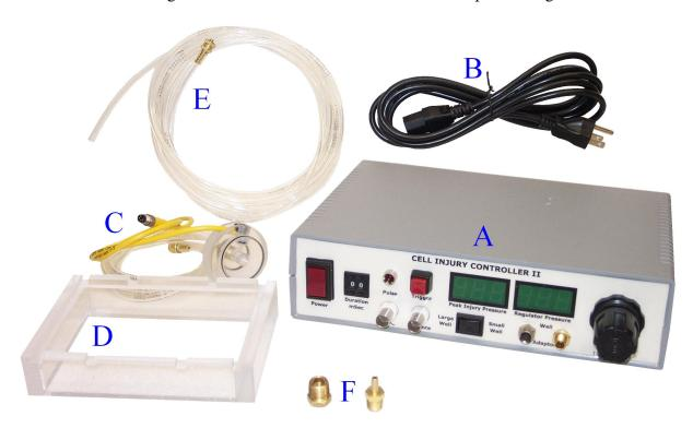
**External Requirements** - The CIC II requires electrical power, a pressurized gas source, and elastic bottomed cell culturing trays.
