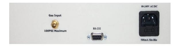
Gas Input - This is the connection for the pressurized gas source. The recommended source pressure is 60 to 80 PSI (414-552 kPa) and should not exceed 100PSI (690 kPa). Gas cylinder pressures are in the thousands of pounds. A tank regulator is required.
